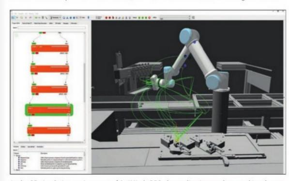
In the 3D simulation environment of ArtiMinds RPS, the application can be tested in advance, checked for collisions and reachability, and individual processes such as greasing and joining can be visualized.
